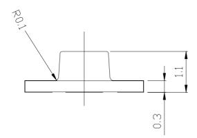
For reflow soldering(Propose)
