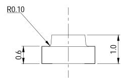
For reflow soldering (propose)
