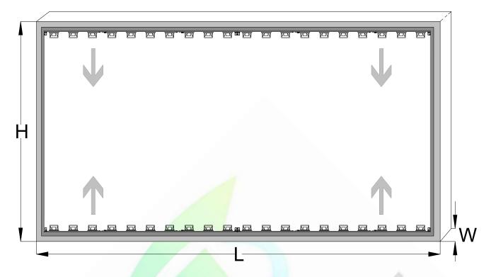
Installation schematic description: the test panel is 3mm thick acrylic white board, and the light transmittance is about 54.4%. Aluminum alloy is selected as the light box model, which is evenly arranged according to the photoelectric performance parameters of the product
