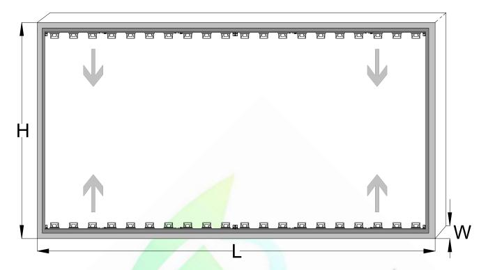
Installation schematic description: the test panel is 3mm thick acrylic white board, and the light transmittance is about 54.4%. Aluminum alloy is selected as the light box model, which is evenly arranged according to the photoelectric performance parameters of the product
