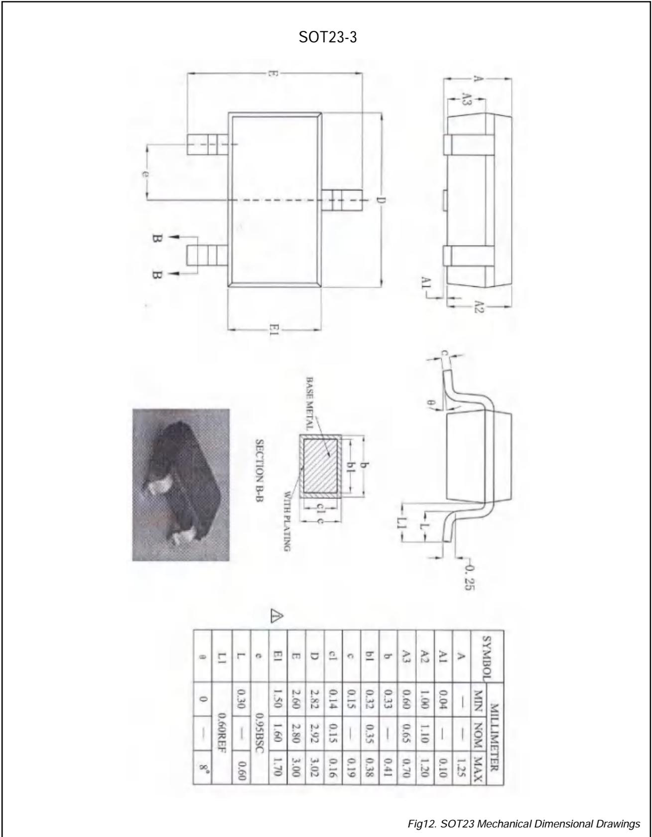
Fig12. SOT23 Mechanical Dimensional Drawings
