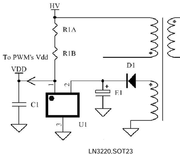
Fig5. Typical resistor start-up system Schematic ( R1A/R1B is the starting resistor of the PWM IC )
