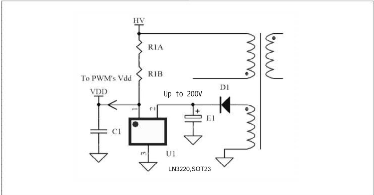
Fig3. Typical Simplified Schematic
