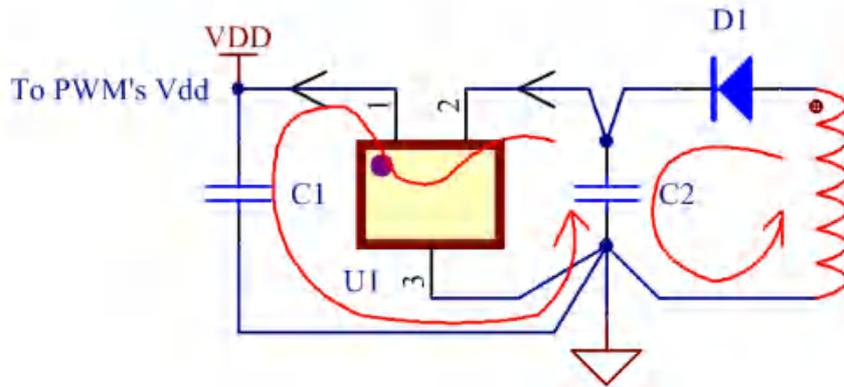
Fig9. Typical PCB Layout loop Schematic
