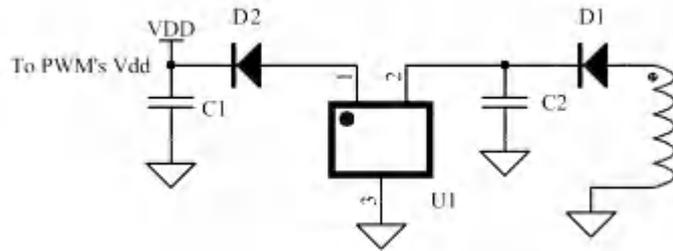
Fig7. Typical circuit connection with reverse isolation.
